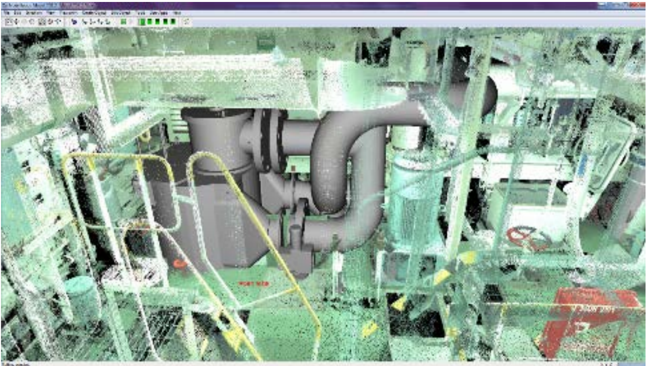
Picture 3: Trojan Marinex fit & connected in vessel
